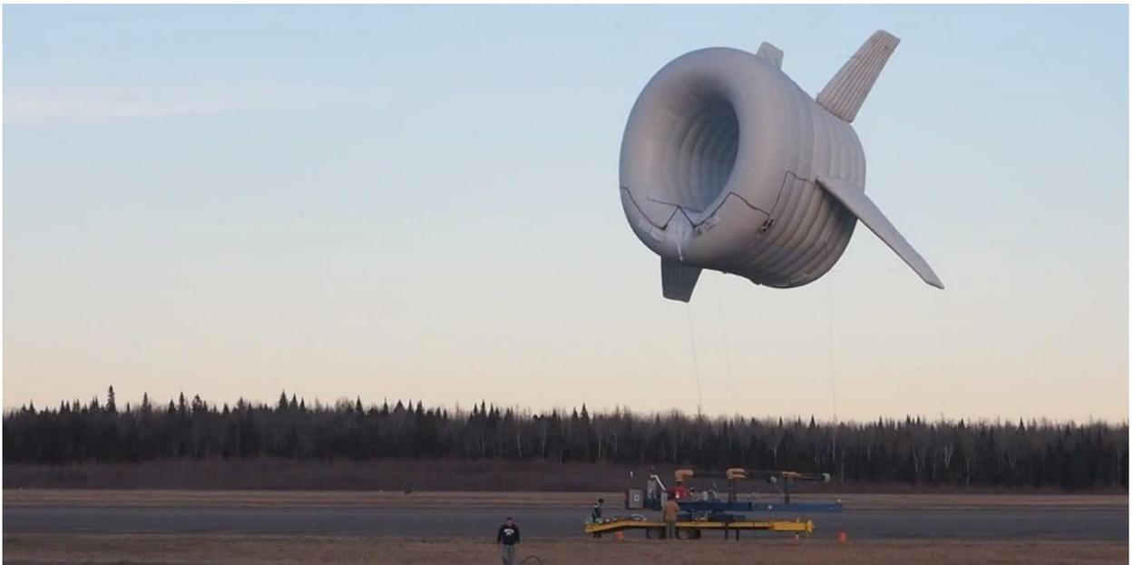
**Figure 4: Movable High-Altitude Wind Turbine**
